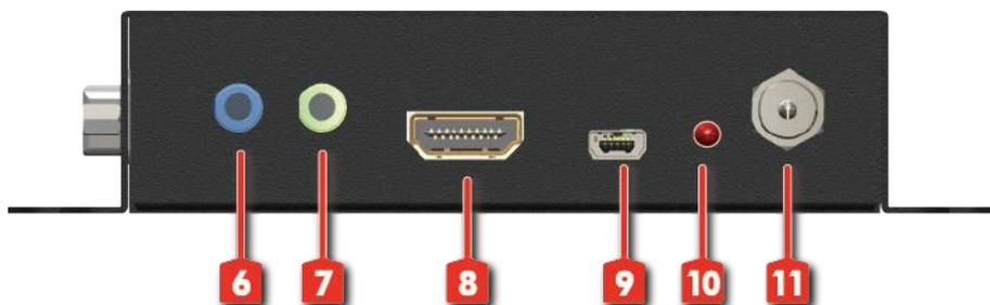
6. **IR Blaster:** Infrared 3.5mm socket for plugging in the extension cable of IR blaster
