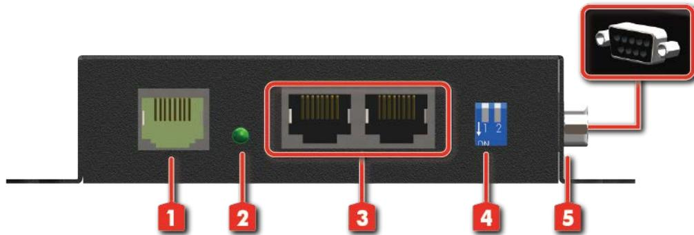
1. **RJ45:** Plug in a Cat-5/5e/6 cable that needs to be linked to the transmitting unit RX.
